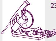
**Electric Powered Railcutter**
